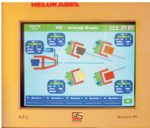
Process control for a large cabling machine at our Windsbach factory.
